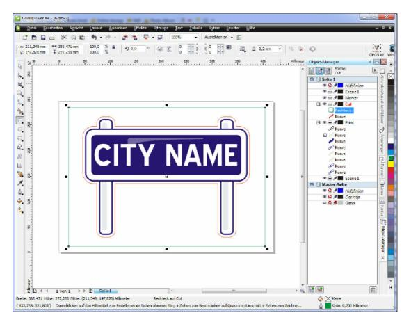
Now must be added the marker. Therefore open the calibration master file and copy one of the marker from here into the actually document.
