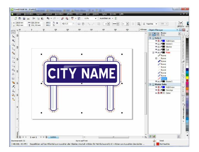
Draw a rectangle which encloses the complete graphic and give it a different, striking color. This rectangle should be left in the level/layer **Cut.**
