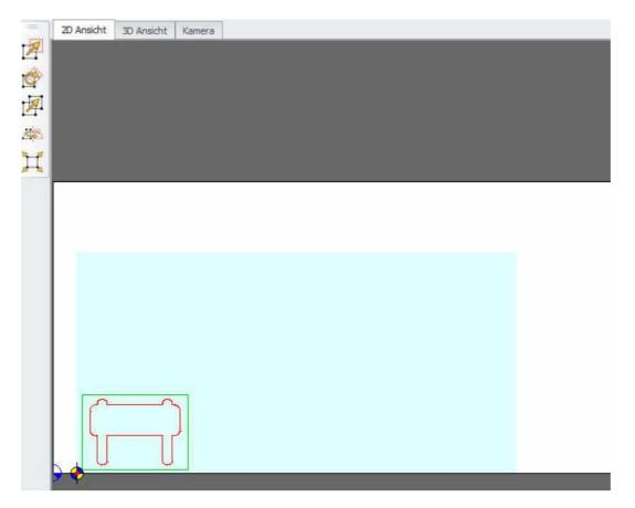
The rectangle around this contour is simple information about the size of sheet only and will be not cut / milled. In the tool box the corresponding tool can be switched out.
