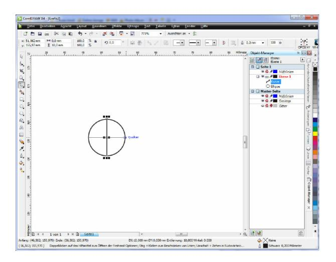
Select all three objects and make a group of them. Hereby you made a marker for the positioning. Now the attributes should be assigned of lines to the marker. Recommendation of the line width is 0.5 mm
