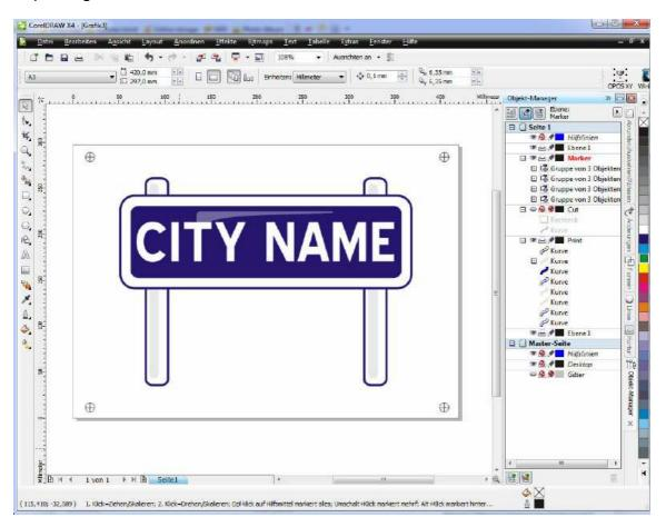
For the cutting/milling data the levels/layers Print and Marker will be switched off.
